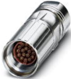
Cable connector, straight, Screw locking, M17, Number of positions: 17, Type of contact: Socket, Crimp connection, shielded: Yes, Cable diameter: 8 mm...10 mm
