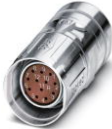
Cable connector, straight, shielded: Yes, SPEEDCON locking, M23, Number of positions: 17, Type of contact: Socket, Crimp connection, Cable diameter: 3 mm ... 14.5 mm
