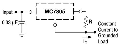
The MC7800 regulators can also be used as a current source when connected as above. In order to minimize dissipation the MC7805C is chosen in this application. Resistor R determines the current as follows:
