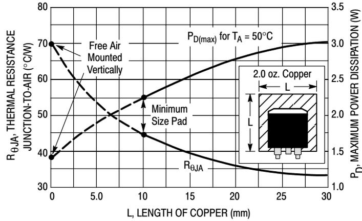
Figure 14. D<sup>2</sup>PAK Thermal Resistance and Maximum Power Dissipation versus P.C.B. Copper Length
