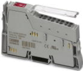
Inline digital output terminal block, complete with accessories (plug and labeling field), 1 relay PDT contact, 5 - 253 V AC, 3 A
