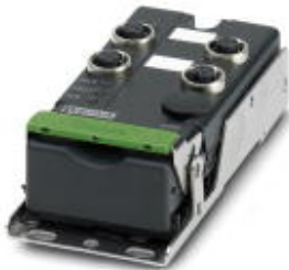
AS-i digital input/output module, AB slave, 2 digital inputs, 24 V DC, 2, 3 and 4-conductor connection method, 2 digital outputs, 24 V DC, IP67 protection
