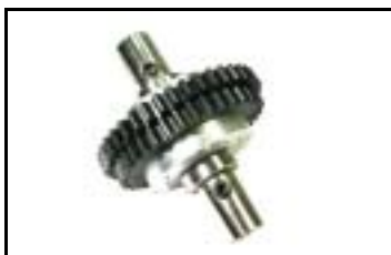
C. Install ball bearing & joint.
