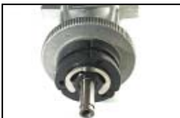
C. Install the fly wheel and clutch shoes.
