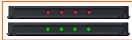
The row of four LED input indicator lights will light up first red then green; this will repeat three times. Then the red light will light up once to determine which slots are in use.
