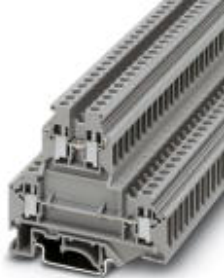
Feed-through terminal block, Cross section: 0.2 mm 2 - 4 mm 2 , AWG: 24 - 12, Connection type: Screw connection, Width: 6.2 mm, Color: gray, Mounting type: NS 35/7,5, NS 35/15, NS 32
