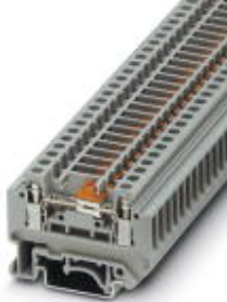
Disconnect terminal block, Connection method: Screw connection, Cross section: 0.2 mm 2 -4 mm 2 , AWG: 24 - 12, Width: 6.2 mm, Mounting type: NS 35/7,5, NS 35/15, NS 32, Color: blue
