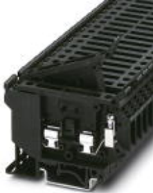
Fuse terminal block for cartridge fuse insert, cross section: 0.2 - 4 mm 2 , AWG: 26 - 10, width: 8.2 mm, color: Gray
