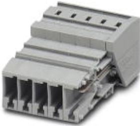
Coupling, Connection method: Spring-cage connection, Number of positions: 2, Cross section: 0.08 mm 2 - 6 mm 2 , AWG: 28 - 12, Width: 12.4 mm, Height: 22.3 mm, Color: gray
