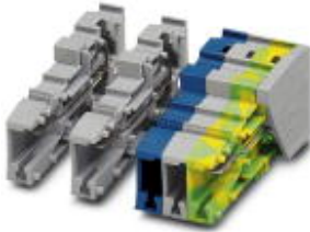
Coupling, Connection method: Spring-cage connection, Number of positions: 1, Cross section: 0.08 mm 2 - 6 mm 2 , AWG: 28 - 10, Width: 6.2 mm, Height: 22.3 mm, Color: green-yellow
