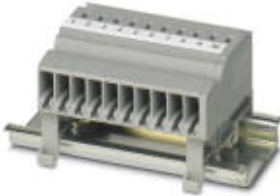
Coupling, Connection method: Plug connection, Number of positions: 10, Cross section: 0.08 mm 2 - 4 mm 2 , AWG: 28 - 12, Width: 52 mm, Height: 18.8 mm, Color: gray
