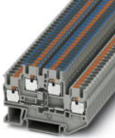
Double-level terminal block, Cross section: 0.14 mm 2 - 4 mm 2 , AWG: 26 - 12, Connection type: Push-in connection, Width: 5.2 mm, Color: gray, Mounting type: NS 35/7,5, NS 35/15
