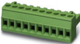
Plug component, Nominal current: 12 A, Rated voltage (III/2): 320 V, Number of positions: 9, Pitch: 5.08 mm, Connection method: Screw connection, Color: green, Contact surface: Tin
