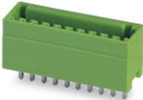
Header, Nominal current: 4 A, Rated voltage (III/2): 160 V, Number of positions: 2, Pitch: 2.5 mm, Color: green, Contact surface: Tin, Assembly: Soldering
