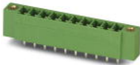
Header, Nominal current: 8 A, Rated voltage (III/2): 160 V, Number of positions: 11, Pitch: 3.81 mm, Color: green, Contact surface: Tin, Assembly: Soldering
