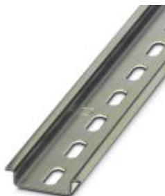
DIN rail, material: steel galvanized and passivated with a thick layer, perforated, height 7.5 mm, width 35 mm, length: 755 mm
