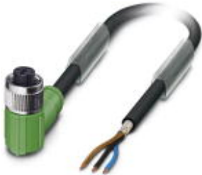
Sensor/Actuator cable, 3-position, PUR halogen-free, Black-gray RAL 7021, shielded, Free cable end, on Socket angled M12, A-coded, Cable length: 5 m
