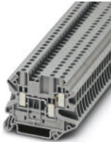
Feed-through terminal block, Connection method: Screw connection, Cross section: 0.14 mm 2 - 4 mm 2 , AWG: 26 - 12, Width: 5.2 mm, Color: gray, Mounting type: NS 35/7,5, NS 35/15
