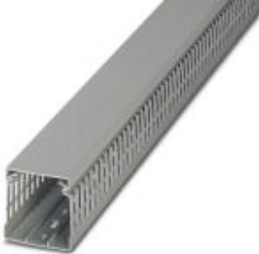
Cable duct, light gray, halogen-free, consisting of upper part and mounting base, width: 25 mm, height: 80 mm, length: 2000 mm
