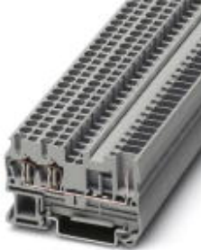
Feed-through terminal block, Connection method: Spring-cage/plug-in connection, Cross section: 0.08 mm 2 - 4 mm 2 , AWG: 28 - 12, Width: 5.2 mm, Color: gray, Mounting type: NS 35/7,5, NS 35/15
