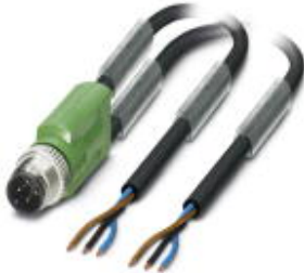
Sensor/Actuator cable, 3-position, PUR halogen-free, Black-gray RAL 7021, Plug straight M12, A-coded, on Free cable end and Free cable end, Cable length: 1.5 m
