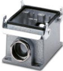
Box mounting base, with double locking latch, height 72 mm, with screw connection, 1x Pg29
