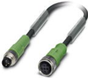
Sensor/Actuator cable, 3-position, PUR halogen-free, Black-gray RAL 7021, Plug straight M8, on Socket straight M12, A-coded, Cable length: 3 m
