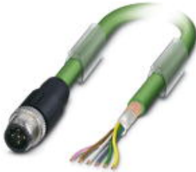
Bus system cable, INTERBUS, INTERBUS, 5-position, PUR halogen-free, Green RAL 6017, shielded, Plug straight M12, B-coded, on Free cable end, Cable length: 5 m
