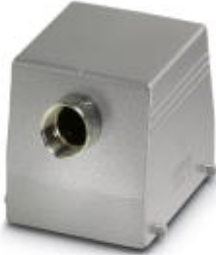
Sleeve housing, for double locking latch, height 80 mm, without screw connection, 1x Pg29, lateral cable entry
