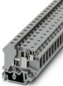
1-level terminal block with double connection on one side, cross section: 0.5 - 10 mm 2 , AWG: 24 - 6, width: 10.2 mm, color: gray
