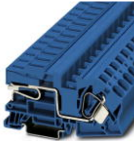
Installation level terminal block, Spring-cage connection, Cross section: 0.2 mm 2 - 25 mm 2 , AWG: 24 - 4, Width: 12 mm, Color: blue, Mounting type: NS 35/15, NS 35/7,5
