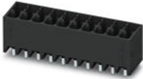
Header, Nominal current: 8 A, Rated voltage (III/2): 160 V, Number of positions: 13, Pitch: 3.5 mm, Color: Black, Contact surface: Tin, Assembly: SMD/THT/THR
