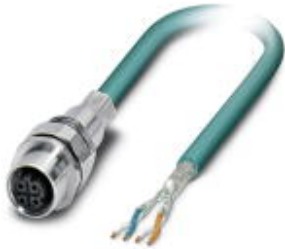
Assembled Ethernet cable, CAT5e, shielded, 2-pair, AWG 26 stranded (7-wire), RAL 5021 (water blue), M12 flush-type socket, front/screw mounting with M16 thread on free conductor end, line, length 2 m
