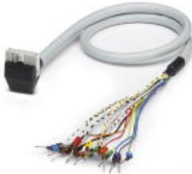
Assembled round cable with a 20-pos. molded socket strip (90° output) and an open end. On the open end, the wires are labeled with 1 to 20 and have ferrules, cable length: 1.5 m
