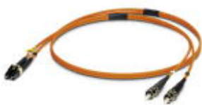
Assembled fiber optic cable, break-out cable, fiberglass multi-mode 50/125 µm, connector: LC/B-FOC (ST), degree of protection: IP20, for installation in cable ducts or control cabinets, length: 2 m
