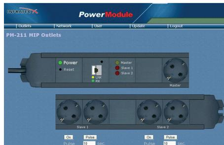
when actually in the office. For example, if the monitor connected to the master socket is switched on, the socket strip automatically detects which consumer devices are connected to the slave connections and then supplies them with power.
